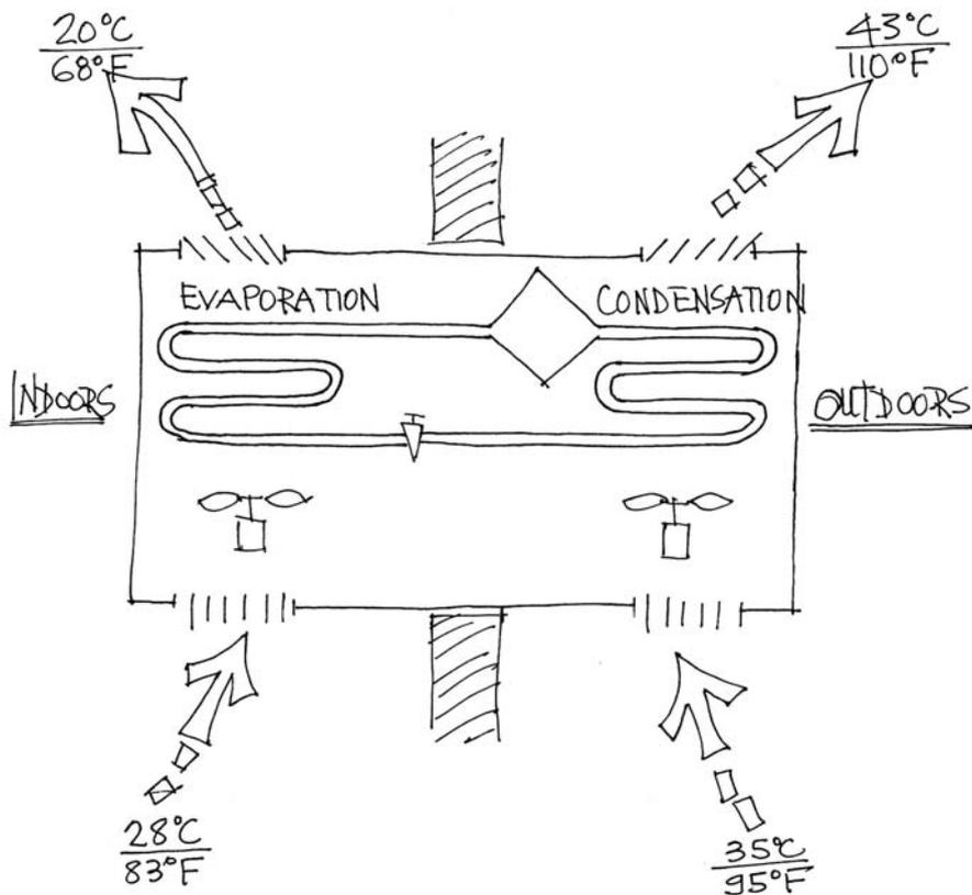
Figs. 5 & 6: Thermal image of individual air-conditioner in cooling mode, ejecting hot air to the urban air; and internal mechanism of refrigerative system indicating how hot air is removed from the inside of the building but not eliminated, being simply transferred to the outside air.
